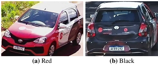
Figure 9. Examples of misclassified multicolored vehicle from different viewpoints. The predicted color is shown below each image. Depending on the camera angle and illumination, a single color can appear dominant, which causes the classifier to classify the vehicle based on that one color.
