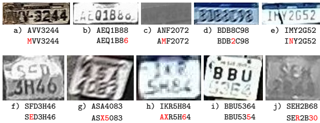
Figure 12. Example of misrecognized LPs. For each image, the ground-truth label is shown above the model’s prediction, with incorrectly recognized characters highlighted in red. The failure cases include severely degraded characters (a, h, i), illumination-induced obstructions (b), low-contrast characters (c, j), blurring (d, g), and physically deformed LPs (e, f).
